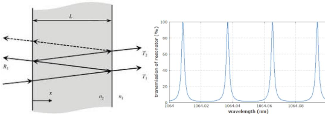
Figure 11.4: (Left) The Fabry-Perot Cavity, displaying the sequence of reflections and transmissions of e-m waves at the two leaky mirrors and (Right) the Transmission coefficient of the F-P cavity as a function the e-m wavelength. Source: The internet.
