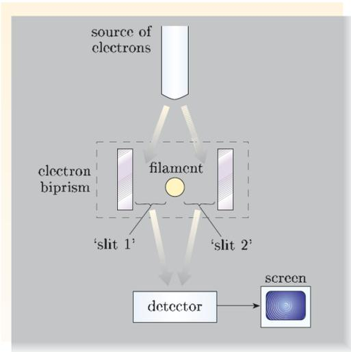
**Figure 1.12** Schematic representation of an experimental arrangement used by Tonomura in 1989 to demonstrate the wave-particle duality of electrons. The two paths of the electrons around the filament are analogous to the paths through two slits in an otherwise absorbing screen.
