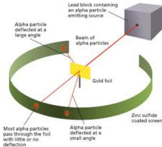
Figure 2.16: A schematic diagram of the experimental setup for the Rutherford gold foil scattering experiment, in which positively charged  $\alpha$  particles (that emerge from the radioactive decay process of the source) are directed at a target thin gold foil. The observation of large-angle scattering provides strong evidence for the existence of a positively charged nuclear core within the atom. Source: The internet.
